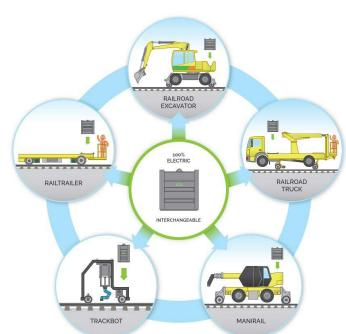
Machines such as excavators, self-propelled rail trailers, and the Trackbot are already equipped with this technology.
