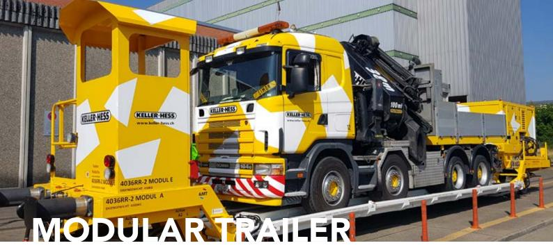
Together with our Swiss partner AMT developed a special railtrailer which is modular for transporting special vehicles or loads on the rail.
