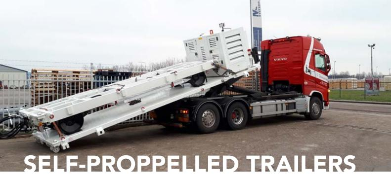
AMT's self-propelled rail trailers are modularly designed. As a result, almost all options are interchangeable with the non-driven rail trailers. The trailers have two or four hydrostatically driven wheels with fail-safe brakes.
