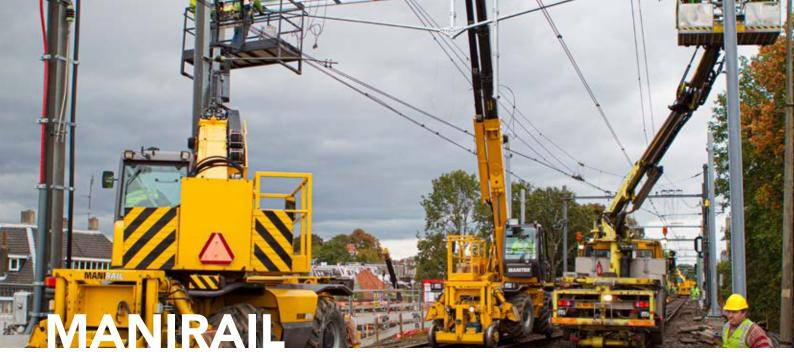
This multi-functional, 360-degree rotating telescope machine offers the user a means of transport, telescopic handler, MEWP and hoisting crane all in one. The compact rail conversion ensures that the machine has a maximum working range. A comprehensive control system with built-in safety and control functionalities provides ergonomic operation.
