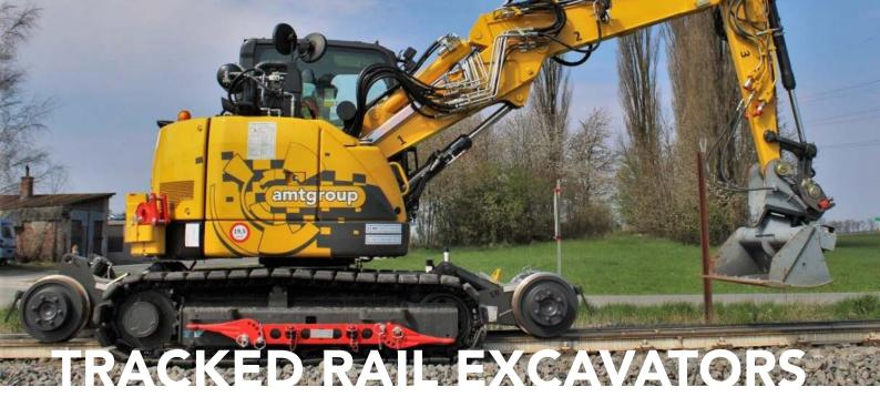
The versatile 85RR (10T) & 145RR (20T) crawler excavators are equipped with a fixed mounted hydraulic rail system. Suited for narrow, normal and tram track with only one wheel swap.
