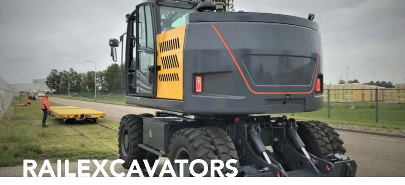
The TW160,165 (20T) and TW180 (22T) are fitted with an extremely stable and robust rail gear system Permanently mounted with optional quick change system for narrow, normal and tram tracks.
